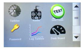
The **Home Screen** for the ECU is displayed. All the functions available can be displayed by using the scroll bar on the right side of this screen
