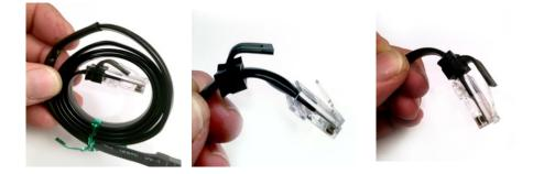
The data connector at the turbine end has a new safety latch and removal assisting mechanism. This assist device pictured above on the left if placed under the plastic tab when attached to the turbine acts as a locking mechanism. The center picture above shows the latch in the retracted position. The picture on the right shows the device above the tab on the data connector in a position to assist with removal of the data cable from the turbine.
