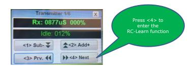
Note: <u>The c</u>orrect reading of throttle % by the ECU can be verified on this screen, percentage of the throttle position is shown on, 0% in the position of engine stop (trim and stick down), 100% with stick/trim full up and between 10% and 30% at idle, (stick up trim down).
