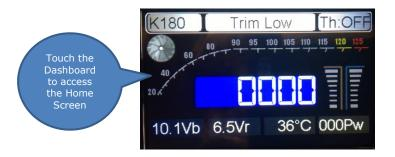
On the Home Screen, touch the Turbine Log to display one of the last four turbine runs or "Rounds".
