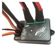
The picture above shows the new single data cable with a keyed connector which prevents it from being inserted into the ECU incorrectly. The picture on the right shows connection of all cables on the ECU from the turbine, receiver, pump and GSU.
