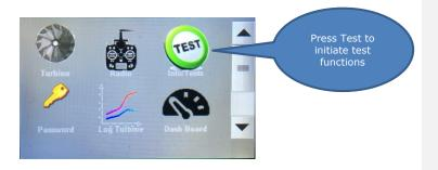
Test/Info page 1 displays Turbine Total Time in minutes, last Cycle time in seconds and number of cycles. *Note: These numbers are reset to 0 upon overhaul. (Interval 25 hours)*
