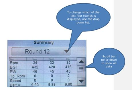
To display all of the information you will need to use the scroll bar on the right side of the screen This information displayed is the Maximum, Mean, and Minimum values for each of the following data items: Turbine RPM EGT - Exhaust Gas Temperature PW Pump Pulse Width Tp\_Rpm (Turbo prop Shaft Rpm) Speed (Air Speed from accessory device) Battery V. : ECU battery voltage RX. V : Receiver battery voltage AMP: ECU current. Engine running only AbNor: Diagnostic Codes
