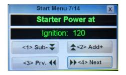
Stage 1 Starter Power: The power sent to the starter motor controlling the amount of air injected into the burner can during the Stage 1.
