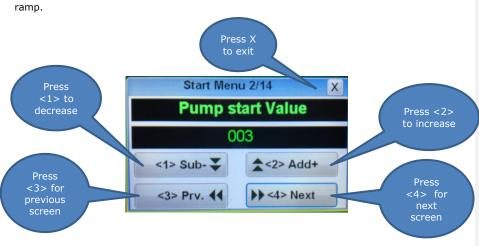
Pump start Value: Sets the power of the pump when it is started at the beginning of the fuel
