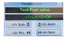
Test/Info page 9 is used for priming the turbine.
